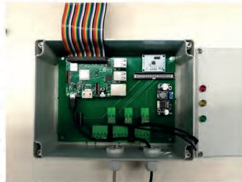
Figure 9 Printed circuit board with Raspberry Pi, real-time clock, analog-to-digital converter and other electronics in grey housing
