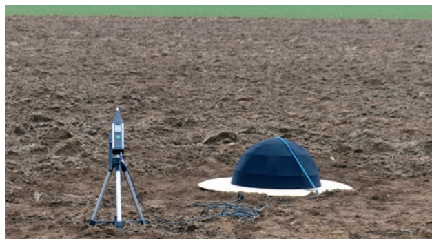
Figure 4.5-3 : Reverberant plate with mounted microphone and dual wind screen. The type DUO measurement device is mounted on a tripod next to it and is connected to the microphone via a measuring cable. Photo: LUBW
