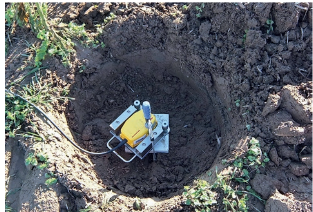
Figure 4.8-2: Vibration measurement point MP D on ground spike at a distance of 285 m from WT 5. Photo: Wölfel company
