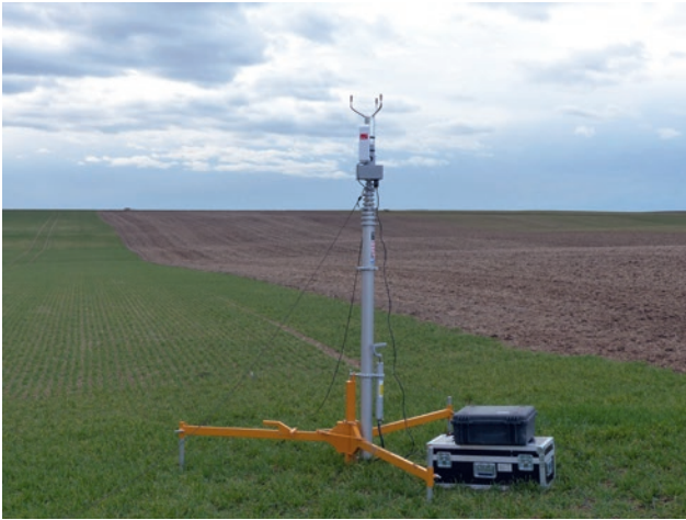
Figure 4.5-4: Anemometer mast for measuring wind speed and wind direction, air pressure, humidity and temperature. The mast is extended to 10 m (not yet extended in the image). Photo: LUBW
